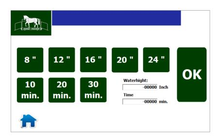
First, select how much water (in cm is to be pumped in. Then select the number of minutes and press "OK" to finish. This takes you to START. If you would like to undo your selection, simply select a different water level and/or time before pressing OK. You can change the settings up until you have pressed OK.
