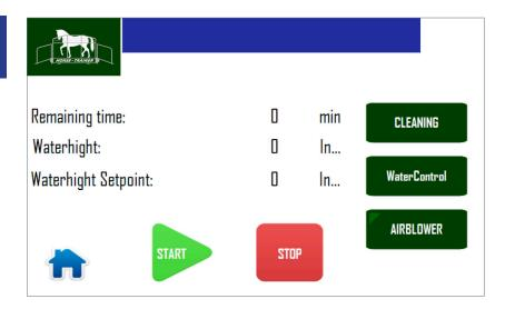
When the CURRENT WATER LEVEL is higher than 15 cm, you can activate the jacuzzi function in the spa by pressing the "AIR JET" button. You can then use the dial to the right of the EMERGENCY STOP to adjust the power of the jets. When the water is pumped out again, the air jets stop automatically once the water surface falls below this level.
