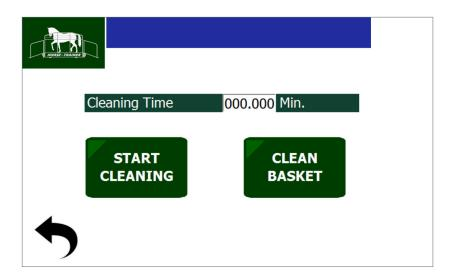
Press "START CLEANING". The equipment will then start pumping water from the tank, through the sand filter and back into the tank. The cleaning program may ONLY be used once all the water is back in the tank.
